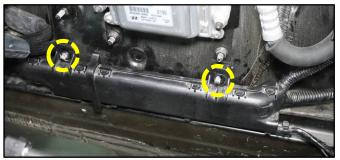
46. Detach the Multipurpose Check connector (W1) from the vehicle and disconnect the A/C Pressure Transducer connector (W2). Detach the wiring harness retaining clip.
