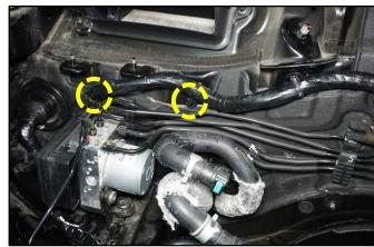
39. Detach the grommet (V4) from the firewall, located behind the ESC module (V2) and pull out connector (D2) removed in step 4 of this procedure.
