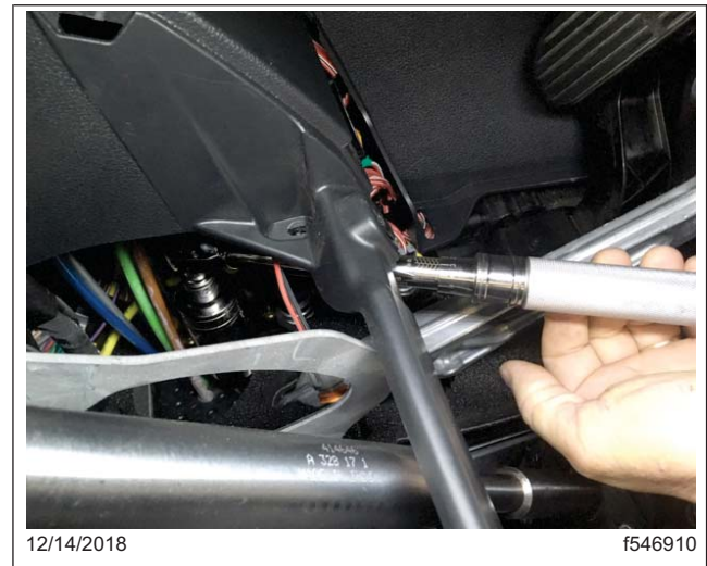
Fig. 3, Tightening the Brake Light Pressure Switch
