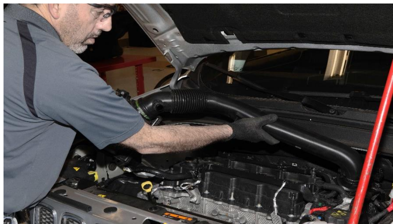
Figure 5 – Air Hose and Housing Assembly
