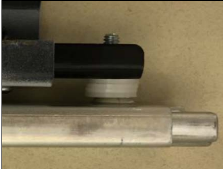
Figure 6: Installed Extension Bracket Connection to the Prop-Rod
