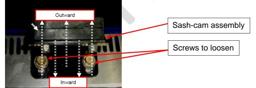
Torque the screws on the sash-cam brackets to 5 Ft-Lbs. until the bracket is solid in position.
