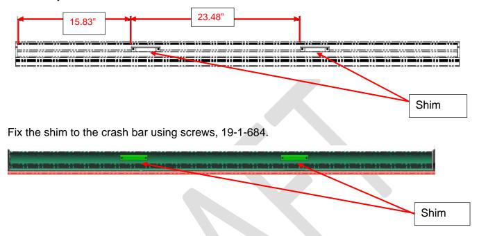
Position the crash bar on the window frame such that there is 0.37" gap between the forward facing edge of the release bar cover and the rear facing edge of the post cover.
