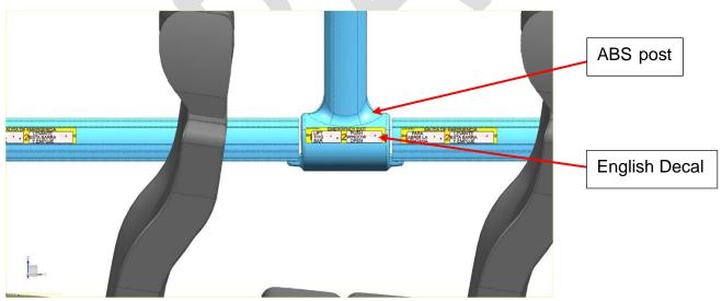
Mark the holes on the post cover and drill 0.12" diameter x 0.37" depth holes.
