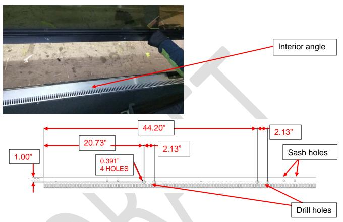
Make the newly drilled holes into 0.547"x0.625" slots into the interior angle only. Be sure not to slot the frame. Install a 19-3-469 rivnut in each slot of the interior angle.
