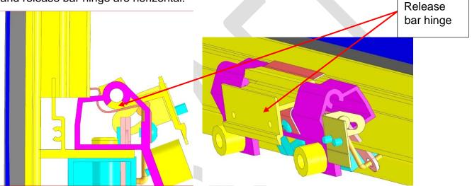
Fix the release bar hinge by inserting the hinge pin, 03-27-1065, through the holes of the latch housing and fasten screws, 03-27-1066, on either ends of the housing to lock the position.
