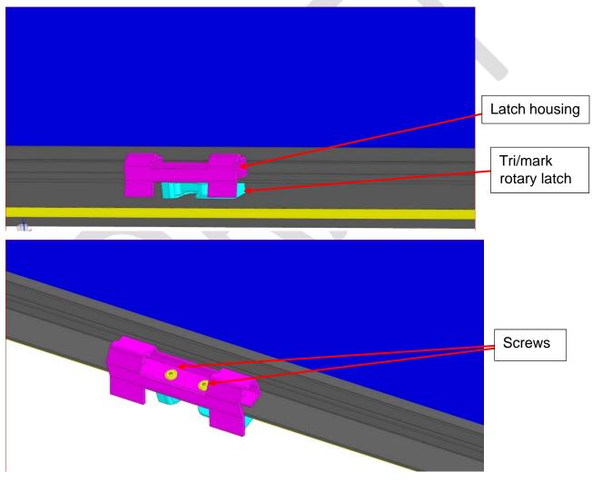
Install the release bar spring, 03-27-1067, to latch housing using screws, 03-27-1914, such that the profile of the spring sits on the profile of the latch housing.
