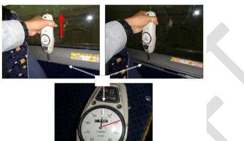
Torque the screws on the sash-cam brackets to 5 Ft-Lbs. until the bracket is solid in position.
