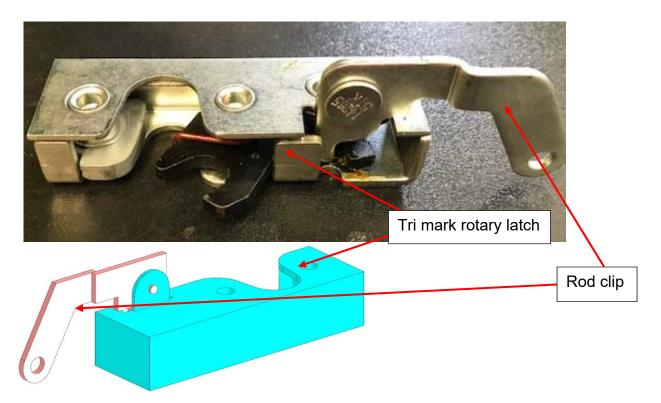
Install formed rod, 03-27-2023, using nylon washers, 03-27-2027, and the release bar bracket, 03-27-2022, as shown in the picture below to the rod clip. Place nylon washers on both sides of the formed rod.
