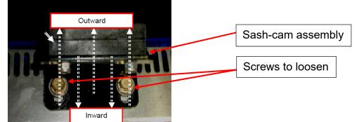
Torque the screws on the sash-cam brackets to 5 Ft-Lbs. until the bracket is solid in position.
