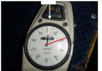
Torque the screws on the sash-cam brackets to 5 Ft-Lbs. until the bracket is solid in position.
