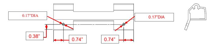
Install a recess bumper, 03-27-1068, at each hole using a screw, 03-27-2033 as shown below.
