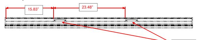
Fix the shim to the crash bar using screws, 19-1-684.
