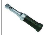
Torque Wrench 1783 2-10Nm -VAG1783-(or equivalent)
