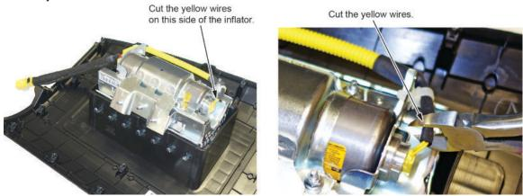
8.2. Strip away about 1 inch of the yellow wire insulation, then twist the wires together.
