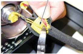
8.3. Strip away about 1 inch of the yellow wire insulation, then twist the wires together.
