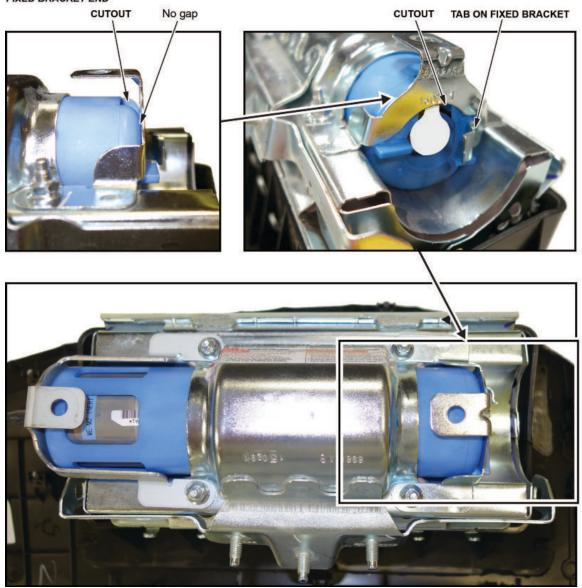
12.3. Install the bracket included in the kit onto the airbag module. There should be no space or gap between the inflator and bracket.
