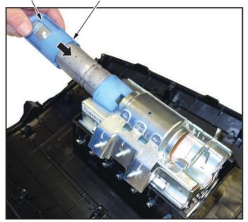
12.2. Slide the inflator in until the plastic collar contacts the bracket. The two tabs should align with the side of the airbag module and the metal tab as shown. There should be no space or gap between the inflator and bracket. There is a red dot located on the fixed bracket side, which may be difficult to see because of the bracket.
