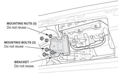
3.4. Remove the mounting nuts from the hook plate.
