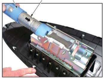
12.2. Slide the inflator in until the plastic collar contacts the bracket. The two tabs should align with the side of the airbag module and the metal tab as shown. There should be no space or gap between the inflator and bracket.
