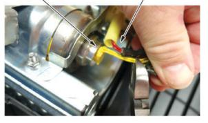
8.3. Strip away about 1 inch of the wire insulation, then twist the wires together.
