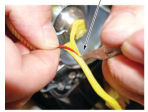
8.2. Cut the yellow wires as shown. Cut the yellow wires on this side of the inflator.
