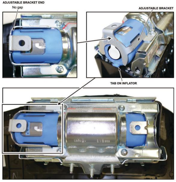
13. Install the new 5 mm locknuts and torque them in sequence to 3.9 N·m (34 Ib-in) . LOCK NUTS (4) 3.9 N·m (34 lb-in)
