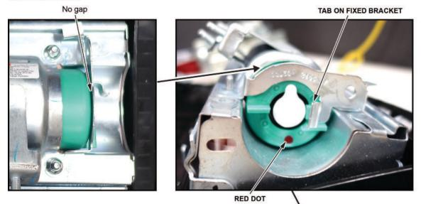
12.3. Install the new bracket included in the kit onto the airbag module. Check there is no space or gap between the inflator and bracket by pushing the bracket against the inflator.
