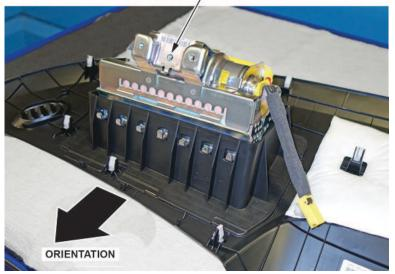
5. Visually inspect the airbag and the inflator for any unusual writing or markings. Refer to IDENTIFYING COUNTERFEIT AIRBAGS.
