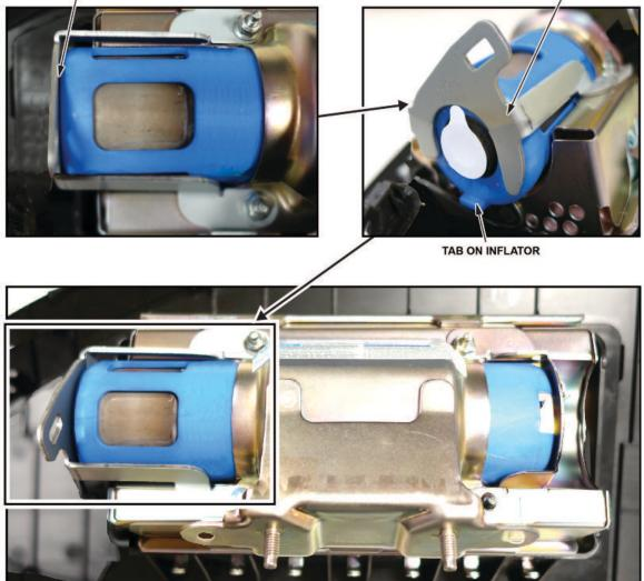
Hold the bracket against the inflator, then install the new 5 mm locknuts and torque them in sequence to 3.9 N•m (34 lb-in).
