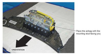
5. Visually inspect the airbag and the inflator for any unusual writing or markings. Refer to IDENTIFYING COUNTERFEIT AIRBAGS.
