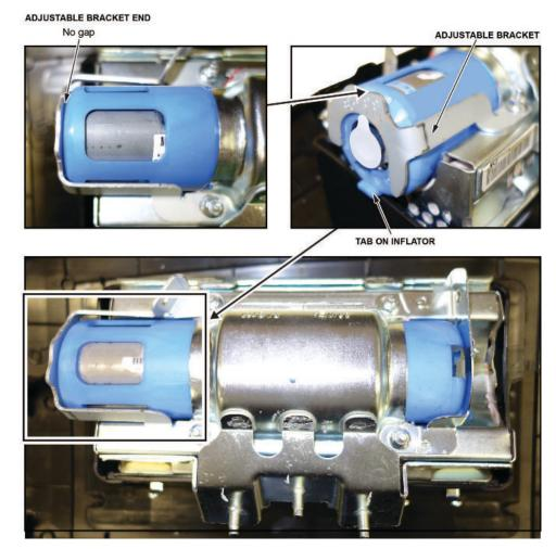
Hold the bracket against the inflator, then install the four new 5 mm locknuts and torque them in sequence to 3.9 N•m (34 lb-in).
