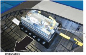
Place the airbag with the mounting studs facing you.
