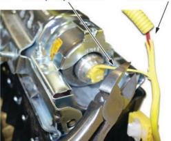
8.3. Strip away about 1 inch of the wire insulation, then twist the wires together.
