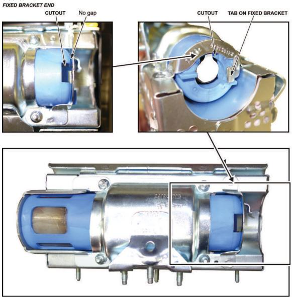
12.3. Install the bracket included in the kit onto the airbag module. Check there is no space or gap between the inflator and bracket by pushing the bracket against the inflator.
