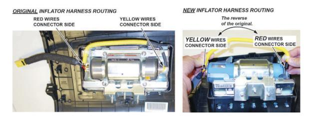
15.2. Connect the red wire connector to the connector on the side with the short plastic collar. Align the "T" shape in the inflator harness connector with the T-shaped inflator connector, then press the connector into place.
