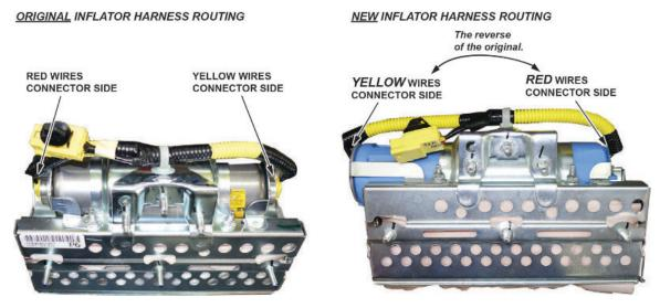
15.2. Connect the red wire connector to the connector on the side with the short plastic collar. Align the "T" shape in the inflator harness connector with the T-shaped inflator connector, then press the connector into place.
