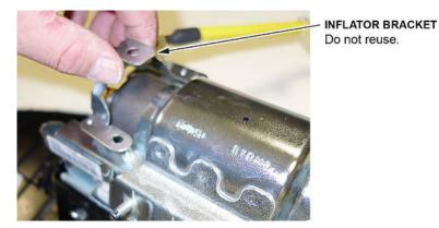
11. Remove the inflator by pushing it out.
