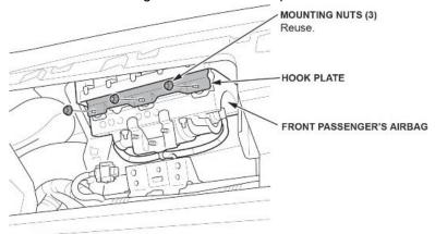
3.5. Release the hooks on the hook plate from the front passenger's airbag housing and remove the hook plate.
