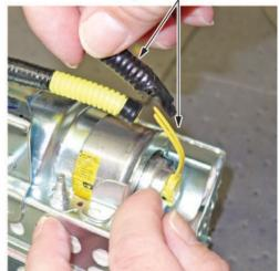
8.2. Strip away about 1 inch of the yellow wire insulation, then twist the wires together.
