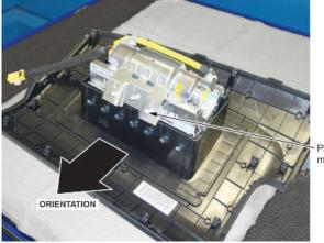
Place the airbag with the mounting stud facing you.
