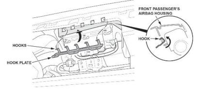
17.3. Install the hook plate with the original mounting nuts.
