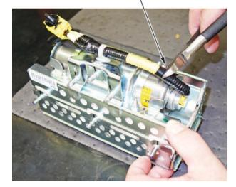
Remove the corrugated tube to expose the yellow wires.
