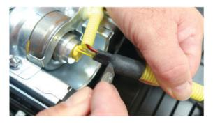
8.2. Cut the yellow wires as shown. Cut the yellow wires on this side of the inflator.
