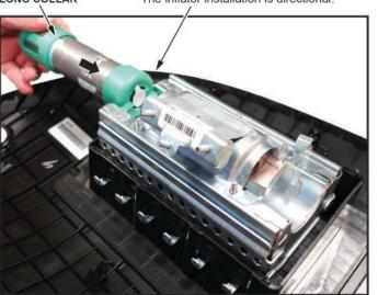
12.2. Slide the inflator in until the plastic collar contacts the bracket. The two tabs should align with the side of the airbag module and the metal tab as shown. There should be no space or gap between the inflator and bracket.
