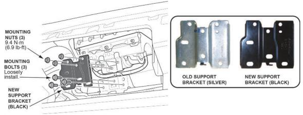
17.5. Push the bracket to the left and hold it while torqueing the mounting bolts to 9.4 N·m (6.9 lb-ft).
