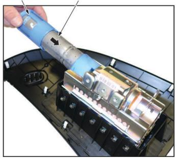
12.2. Slide the inflator in until the plastic collar contacts the bracket. The two tabs should align with the side of the airbag module and the metal tab as shown. There should be no space or gap between the inflator and bracket.
