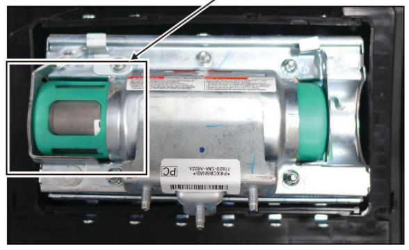
Hold the bracket against the inflator, then install the new 5 mm locknuts and torque them in sequence to 3.9 N•m (34 lb-in).
