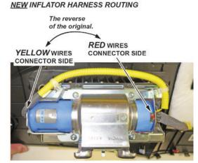
15.2. Connect the red wire connector to the connector on the side with the short plastic collar. Align the "T" shape in the inflator harness connector with the T-shaped inflator connector, then press the connector into place.
