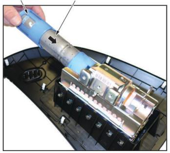
12.2. Slide the inflator in until the plastic cutout and the small flat spot align with the tab on the bracket. There should be no space or gap between the inflator and bracket. There is a red dot located on the fixed bracket side, which may be difficult to see because of the bracket. *FixED BRACKET END*
