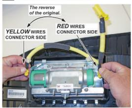
15.2. Connect the two connectors. Align the "T" shape in the inflator harness connector with the T-shaped inflator connector, then press the connector into place.
