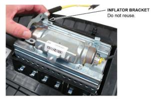
11. Remove the inflator by pushing it out.
