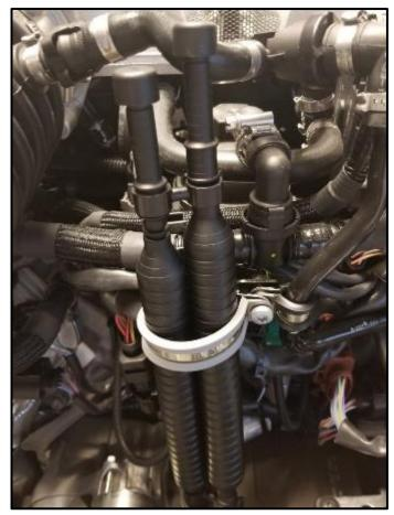
• Carefully remove the oil reservoir cover <1> in direction of <arrows>. Do not jerk or pull it to one side.
