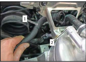
• Make sure the ventilation hose <1> is connected to the transmission.
