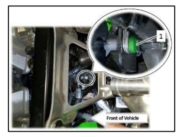
• Remove and discard clips <1> from wiring harness <2>.
