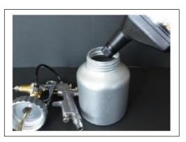
(7) Tighten the lid on the container.Caution: Confirm that the gasket is attached to the lid.
