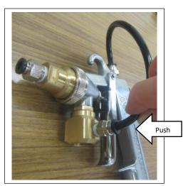
To remove the tube, pull the black part of the air inlet. (When the black part is pressed, the internal teeth are hidden, and when the fingers are released, the teeth appear)
