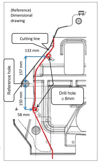
4) Along the drawn line, trim the under cover using Lasha scissor, electric cutter, etc. And drill 2 8mm holes.
