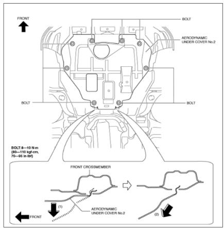
(2) Cut the under-cover to prevent interference with the Side member bracket.1) Cut bold line that includes hole of "Under cover cutting sheet" provided to dealers. Do not throw away the template. There are 3 copies in case one gets damaged.
