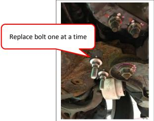
1) Before installing the modified bolt, turn the nut counterclockwise and turn it until it does not turn.
