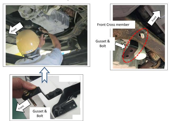
(3) Attach the washer and bolt as shown in the figure and tighten Side member with the specified torque.
