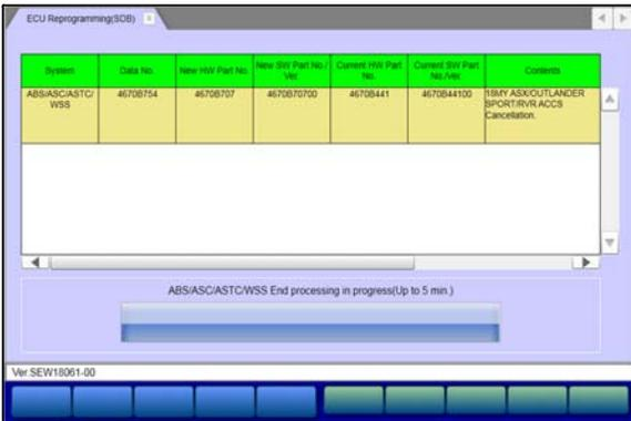
**NOTE: Do NOT disturb the cables or turn off the ignition during reprogramming.**
