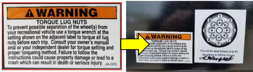
Lug nut torque pattern and warning label
