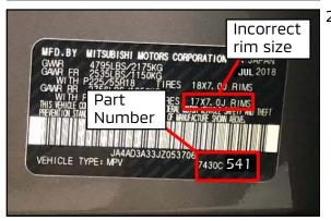
Confirm if the part number on the original label is "7430C**541**" and the rear wheel rim size is "17X7.03."
