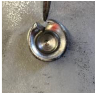
OK Rivet with 1 crack
