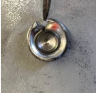
OK Rivet with 1 crack
