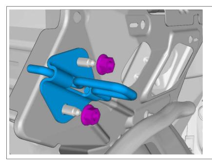
Install the marked component. Install the nuts **Torque:** M10 , 50 Nm
