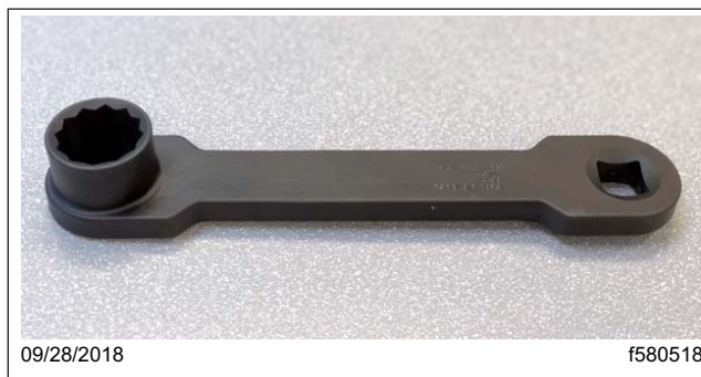
Fig. 1, DDC DSNCHA018005 30mm Air Disc Brake Caliper Brake Bolt Torque Adaptor
