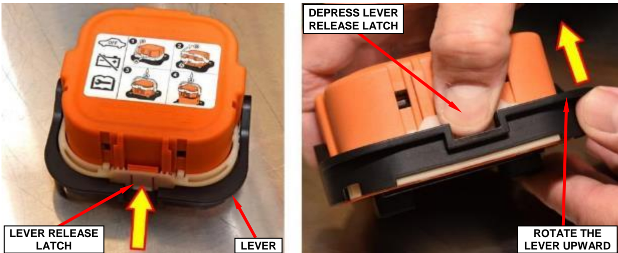
Figure 14 – High-Voltage Manual Service Disconnect First Stage Latch Release (High-Voltage Manual Service Disconnect Removed from Vehicle for Visual Clarity)
