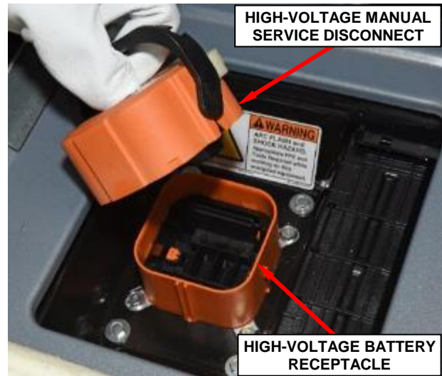
Figure 16 – High-Voltage Manual Service Disconnect and Receptacle
