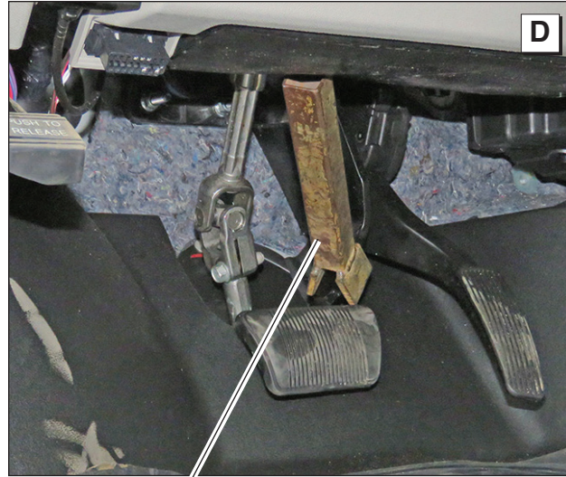
Brake Pedal Blocked
