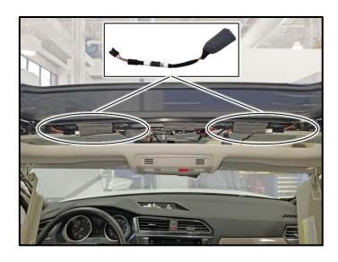
• Install in-line fuses for the left and right panoramic roof ambient light LED modules.
