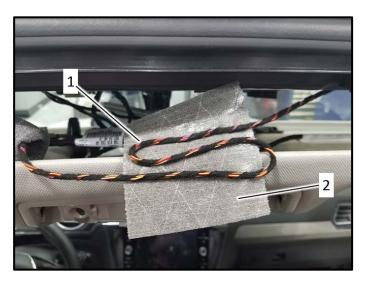
Coil the extra length of harness <1> as shown and secure to the sunroof frame using a foam pad <2>.
