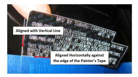
• Once the overlay is properly positioned, apply it fully using your thumb, starting at the bottom edge and working back and forth from the bottom upward to avoid trapping air.
