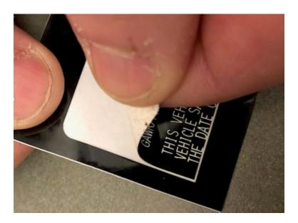
**IMPORTANT NOTE:** The adhesive on the overlay is **YERY** strong. Take the time to confirm the overlay is properly positioned before application as it **will** be destroyed if any attempt is made to remove it.
