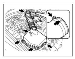
d. Install the air cleaner cap and hose with 4 clamps and the hose clamp.
