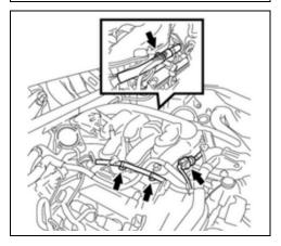
h. Engage the 4 wire harness clamps onto the intake air surge tank.
