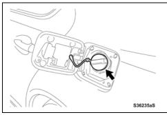
f. Remove the fuel tank filler cap.
