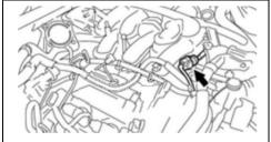
g. Connect the main electrical connector for the fuel injectors at the front of the intake air surge tank.
