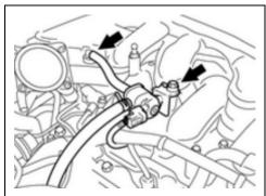
j. Install the No. 1 vacuum switching valve and hose to the intake air surge tank.
