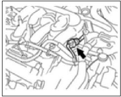
d. Unplug the electrical connector for the LH fuel injectors at the front of the intake air surge tank.
