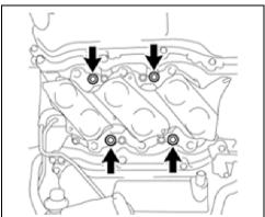
g. Remove the 4 spacers from the intake manifold.
