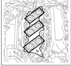
j. Cover the air intake openings to prevent foreign objects from falling into the intake manifold.
