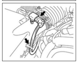
b. Disconnect the MAF sensor connector and harness from the holder.
