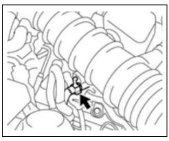
c. Disconnect the ventilation hose from the air cleaner hose clamp.
