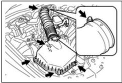
d. Disengage the 4 clamps, loosen the hose clamp, and remove the air cleaner cap and hose.
