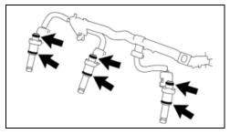
f. Remove the 2 O-rings from each of the 6 fuel injectors. Discard these 12 O-Rings.
