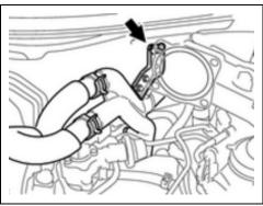
f. Remove the bolt from the RH surge tank support brace.
