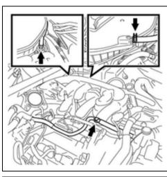
c. Disconnect the ventilation hose, check valve union, and water by-pass hose.
