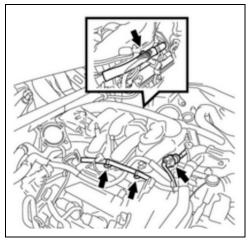
e. Remove the 4 wire harness clamps from the intake air surge tank.
