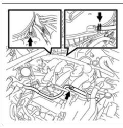
i. Connect the ventilation hose, check valve hose union, and water bypass hose.
