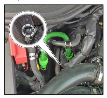
Remove nut <circle> from wiring harness bracket.
