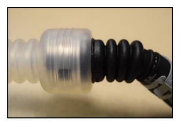
When correctly seated, the fuel line coupling cover should appear as shown.
