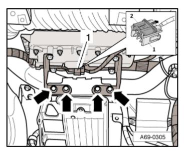
Install new bolts <arrows> on central tube and torque to 9 Nm.
