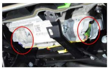
If the passenger airbag inflator connectors are configured on the ends <as shown>, the airbag was manufactured by Takata and will require replacement.
