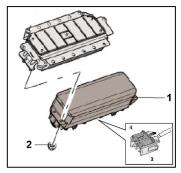
Before handling pyrotechnic components (for example, disconnecting the connector), the person handling it must "discharge static electricity". This can be done by touching the door striker, for example.
