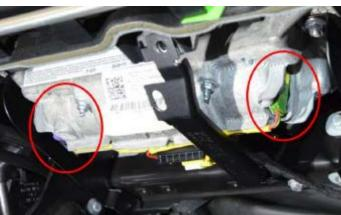
If the passenger airbag inflator connectors are configured on the ends <as shown>, the airbag was manufactured by Takata and will require replacement.
