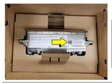
Scan the data matrix code <arrow> of the new airbag at a distance of about 15 cm, then follow the instructions on screen.
