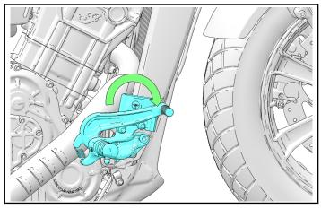
4. Clean and remove reservoir cap on the master cylinder.
