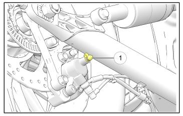
2. Loosen the rear foot control fastener so the foot control can be rotated.
