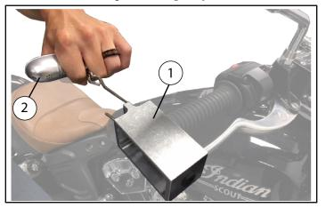
4. Keep tool centered so it does not touch hand grip. Pull on scale connected to tool eyelet.
