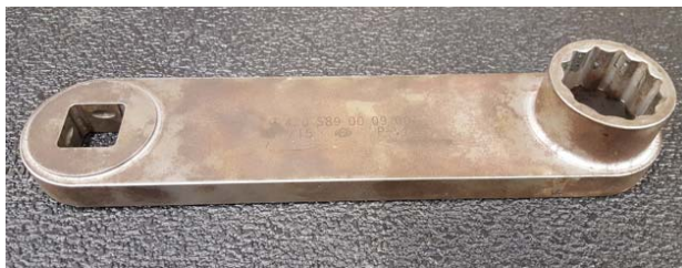
Torque Compensation with Meritor Extension Tool 3256B1354*
