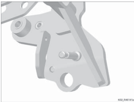
Figure 4: G 310 GS new bearing support for the side stand. (Part number: 46 51 9 480 423)
