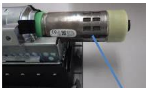
Align guide line (Black line) with retainer edge.
