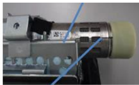
Align guide line (Black line) with retainer edge.
