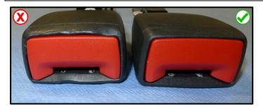
The housing is deformed on the top in the area of the release button.
