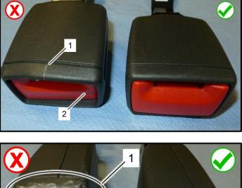
The housing is deformed and/or cracked <1>. •
