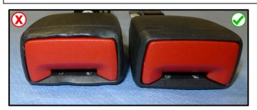
The housing is deformed on the top in the area of the release button.
