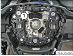
8. Installing the steering wheel
