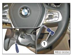
Insert the Torx screwdriver T25 (1) diagonally upwards in the hidden opening on the rear side of the steering wheel until a springing kind of resistance can be felt.
