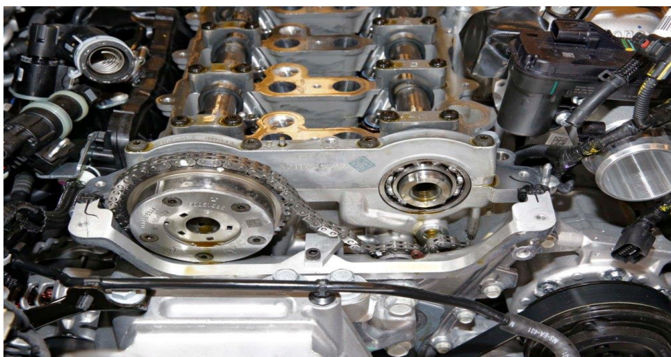
Figure 24 – Intake Cam Phaser Removal
