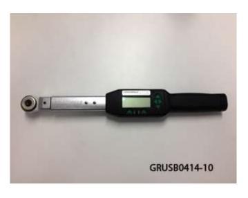
NOTE: Torque the new idler pulley bolt with a digital torque/angle wrench. Use PN 81 64 0 418 185 (automatic tool shipment B04 08 14) or an equivalent type digital torque/angle wrench. To order an additional 0 418 185 torque wrenche contact:
