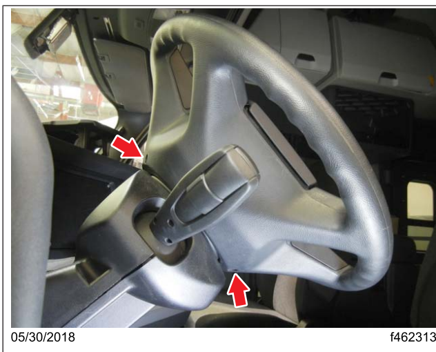
Fig. 1, Locations of the airbag Retainer Screws with the Steering Wheel Turned 90 Degrees
