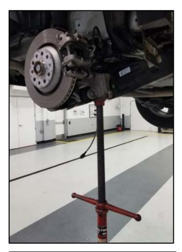
Support the wheel bearing housing with a screw jack so the trailing arm to wheel bearing housing bolt holes align.
