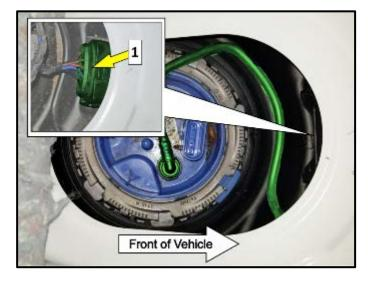
Connect Fuel Pump Control Module -J538-
