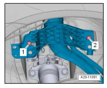
Install new fuel filler neck bolts <1 and 2> and torque to 8 Nm + 90°.
