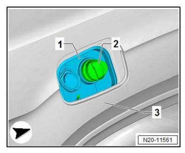
Install the sealing cover <1> into the body <3>.
