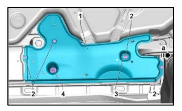
• Install the front and rear underbody trim panels and torque fasteners to 2.0 Nm.
