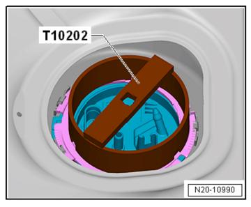
With the aid of a second technician install the locking ring using the -T10202- and torque to 110 Nm.
