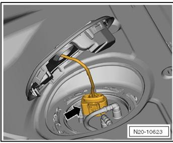
Release and remove the connector <arrow> from the sealing flange.
