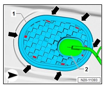
• Unclip the sealing flange cover <1> at the retainers <arrows>.
