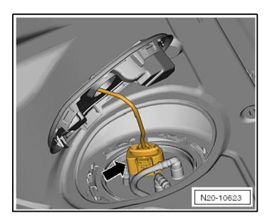
• Connect the connector <arrow> to the sealing flange.
