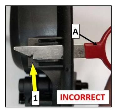
If the Radio Removal Tool -T10057- <A> is inserted over retainer <1>, the locking tabs will not fully release.
