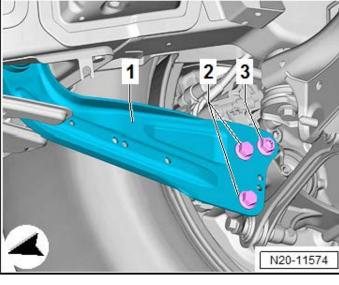
Remove the bolts <2 and 3> and pivot the trailing arm <1> downward.
