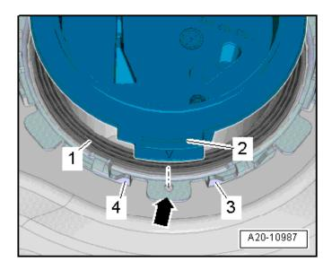
Install the dry fuel delivery unit seal <1> into the opening in the fuel tank.
