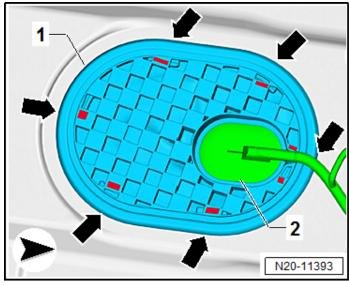
• Install the sealing flange cover <1>.
