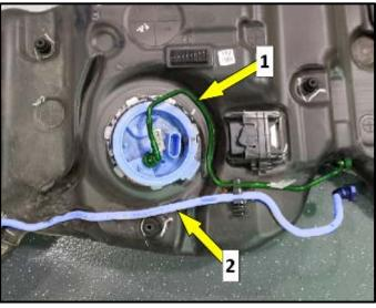
• Transfer fuel line <1> and vent line <2> to the new fuel tank.
