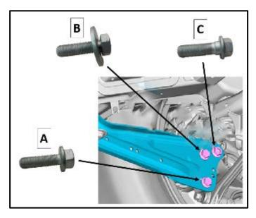
• Install the following bolts in their respective locations and torque to 70 Nm + 90°.
