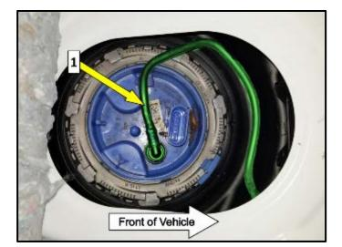
Release and remove the connector <arrow> from the sealing flange.
