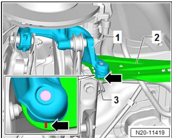
• Support the wheel bearing housing with a screw jack so the trailing arm to wheel bearing housing bolt holes align.
