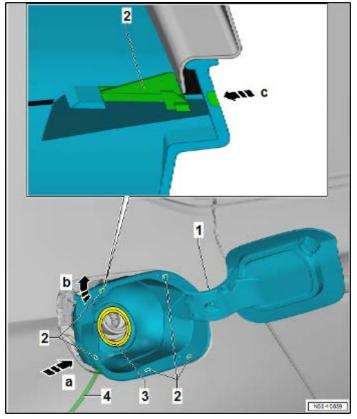
• Install the sealing cover <1> into the body <3>.
