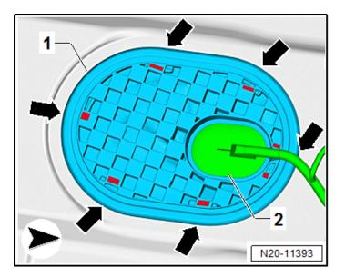
Unclip the sealing flange cover <1> at the • retainers <arrows>.
