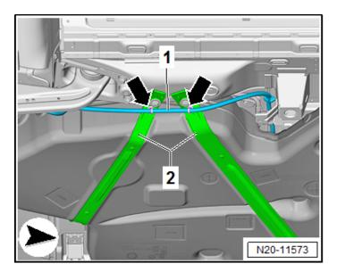
Clip the wiring harness <1> on the mounting straps <2> <arrows>.
