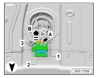
Note the installation position of the fuel line and vent line.
