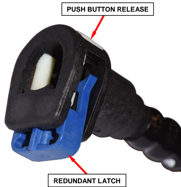
Figure 11 – Fuel Tube Quick-Connect Fitting
