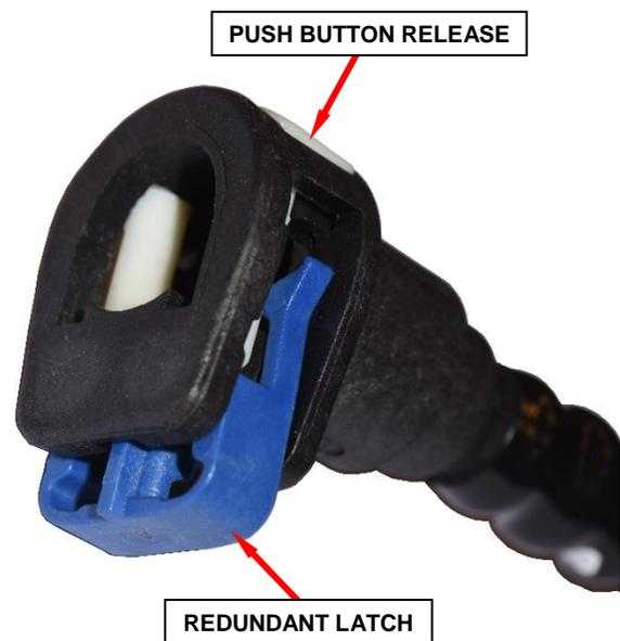
**Figure 11 – Fuel Tube Quick-Connect Fitting**
