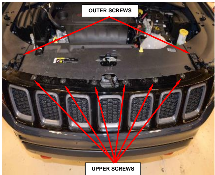
Figure 6 – Upper Fascia Screws
