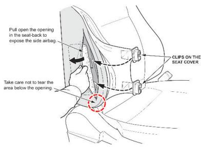
5.2. Pull the side airbag far enough to access the two clips on the seat frame, then attach the clips on the seat cover.
