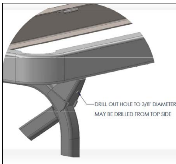
Figure 16: Drilling Location Seat Frame
