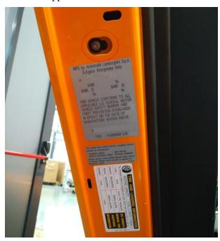
3. Apply three heat reading stickers to monitor the temperature on the entire surface of the label.
