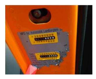
5. Completely remove the label and clean the surface with a soft cloth and a degreaser to eliminate all glue residue.
