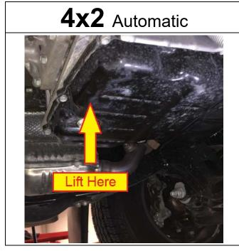
Note: Lift only on the rear most edge of the pan. Lifting in the center of the pan may cause damage.
