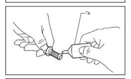
c. Apply sealant to all 3 **NEW** pump housing bolts.
