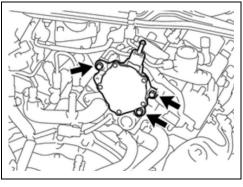
a. Remove the 3 bolts then carefully slide the pump rearward.
