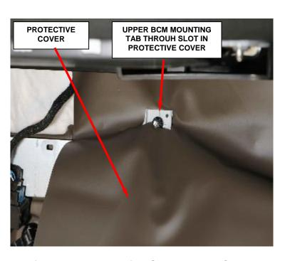
Figure 24 - Protective Cover Over BCM Tab
