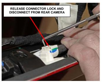
Figure 35 - Rear Camera Connection
