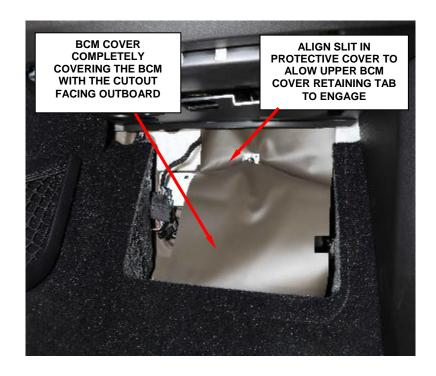
Figure 25 – Protective Cover Installed
