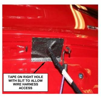
Figure 29 - Cloth Tape to Right Side of Liftgate
