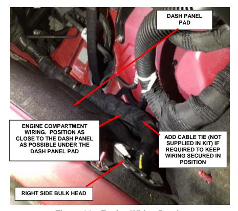
Figure 14 – Engine Wiring Routing
