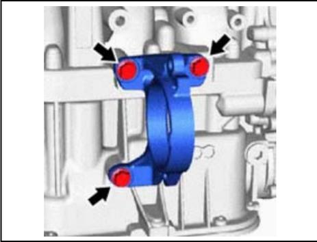
**6. TRANSFER DRIVE SHAFT BEARING BRACKET**
