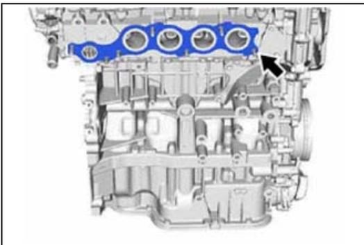
d. Install a **NEW** exhaust manifold gasket onto the **NEW** engine.
