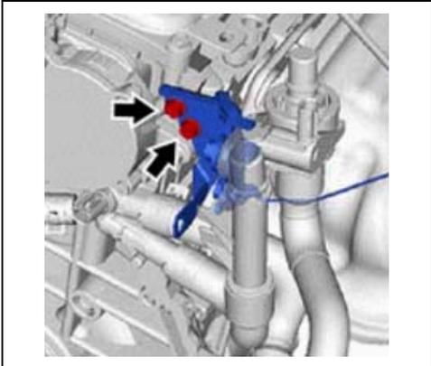
b. Remove the 2 bolts and the water hose bracket.
