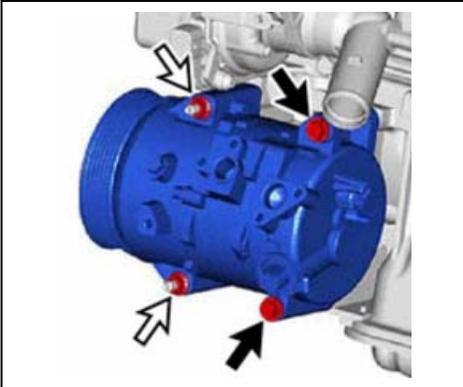
**7. TRANSFER COMPRESSOR ASSEMBLY (type A)**
