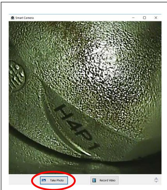
Note: **If the picture starts to turn pink**, the camera is getting too hot. Remove the camera and allow more time for the engine to cool down. The image quality of the camera should return to normal as the camera cools down.
