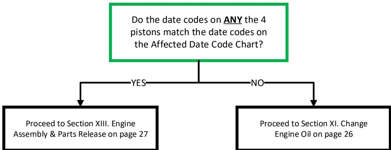
**Help:** In the example above, the piston date code shown is H4P1, which does not match any of the date codes listed on the Affected Date Code Chart. Therefore, this piston is ok. Continue to check the other 3 pistons in the engine against the chart and follow the flowchart for the next step.
