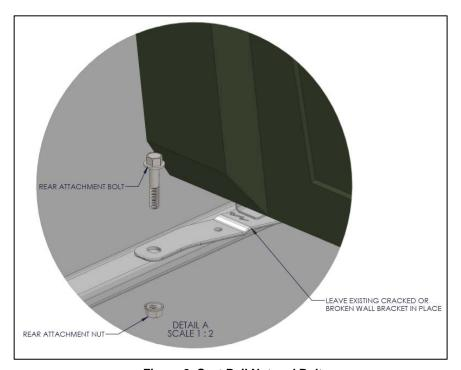
Figure 2: Seat Rail Nut and Bolt
