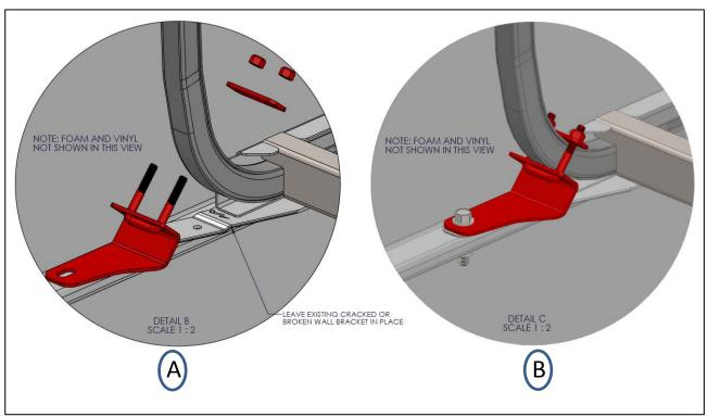
Figure 3: Addition of the New Bracket
