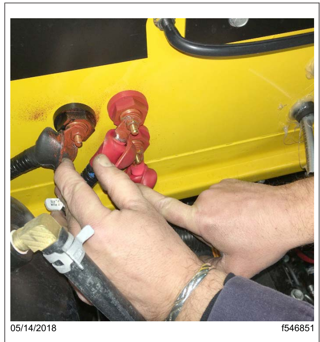
Fig. 2, Removing Connector Protective Cover
