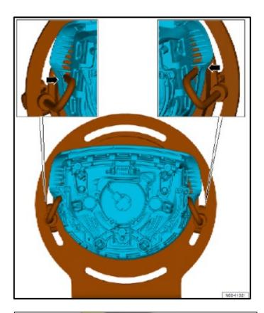
Clamp airbag centrally in airbag support. Securing points on the sides <arrows> and parallel, opposite each other.
