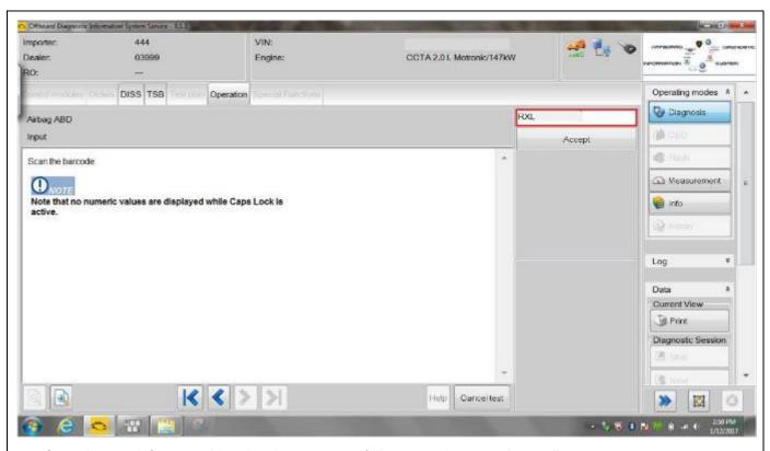
Once the new inflator or airbag has been successfully scanned, press "Accept"
