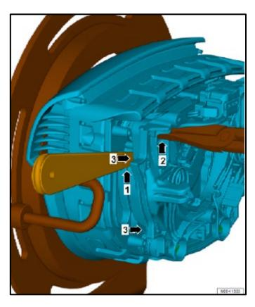
Apply removal wedge -3409- between horn ring and inflator <1> and press together locking elements using longnose pliers <2>.
