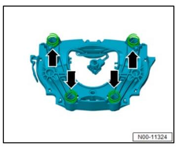
Fit springs <arrows> for horn ring again if necessary.
