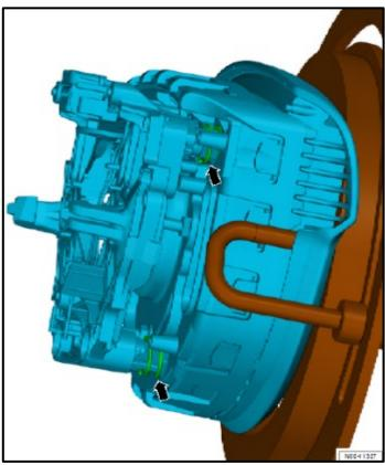
Position horn ring with springs on securing clips and press firmly in place. Ensure that springs are seated correctly on both sides <arrows>.
