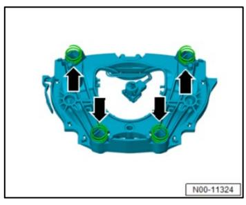
Fit springs <arrows> for horn ring again if necessary.
